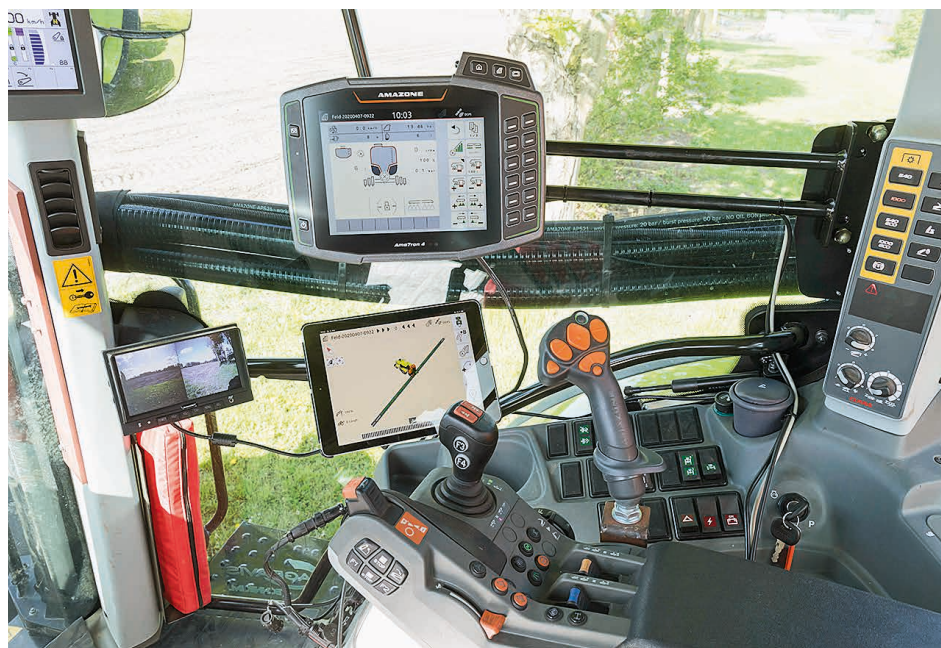
The full spec - Amatron 4, iPad and AmaPilot+ joystick. The camera is located on the left side of the front tank and uses a separate display.
