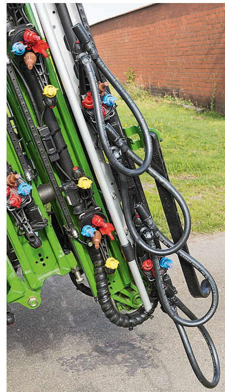
The dribble hoses articulate so they do not stick out to the side. There is now the option of 25cm nozzle spacing.
