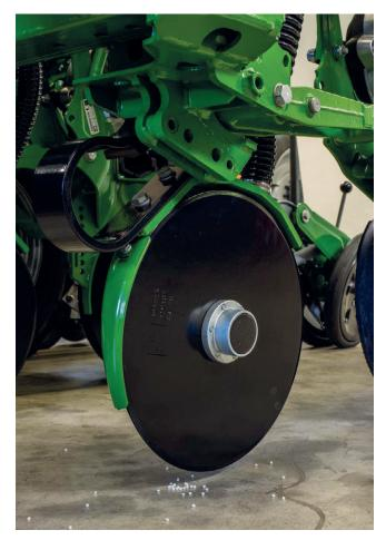
Figure 6: The FerTeC double-disc coulter for fertiliser
