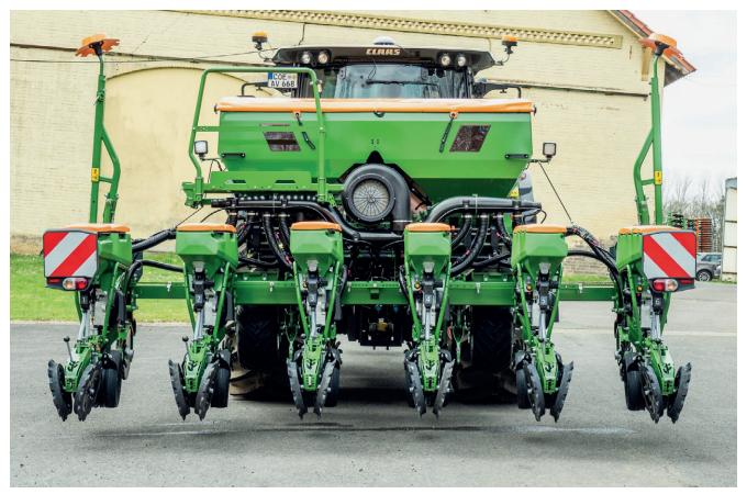
Figure 2: The sowing units in working position
