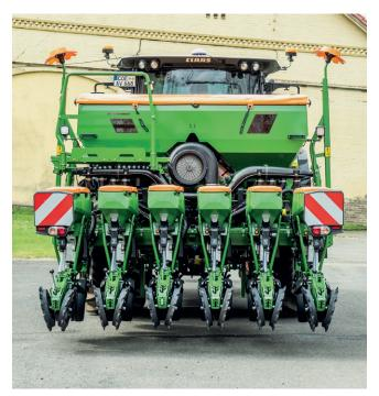
*Figure 3: The sowing units in transport position*
